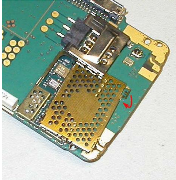
Figure 77 Bending the lock pin and the area around it
