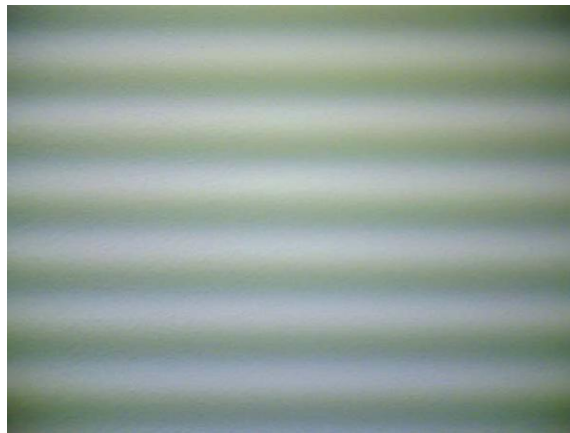
Figure 84 Flicker in an image; object illuminated by strong fluorescent light
