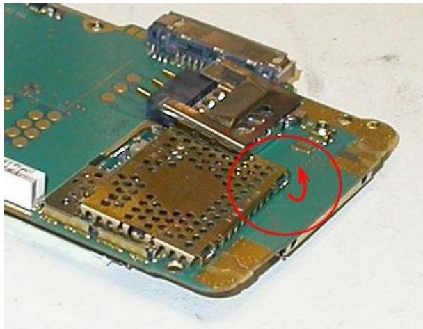
Figure 72 Bending the lock pin and the area around it
