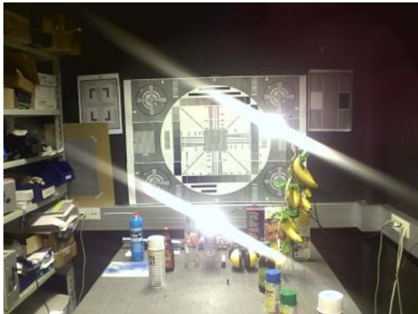
Figure 92 Image of point light sources taken with a dirty (finger print) protective window
