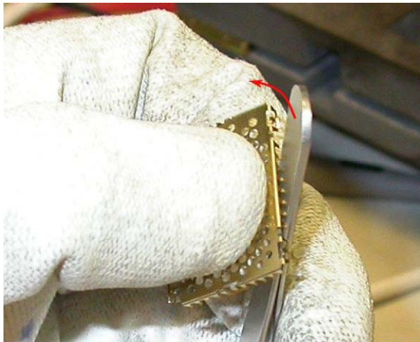
Figure 76 Squeezing the sides of the shield lid
