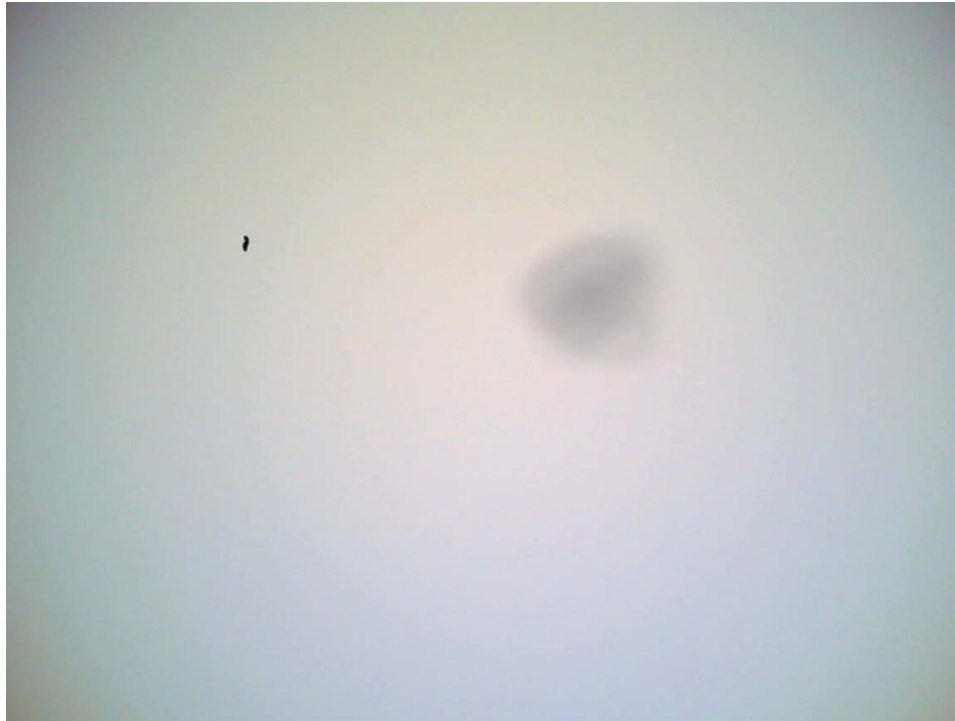
Figure 88 Effects of dust on optical path
