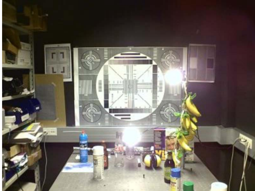
Figure 91 Image of point light sources taken with a clean protective window
