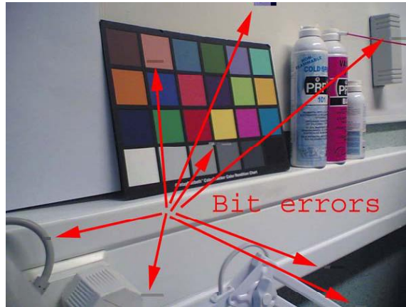
Figure 93 Bit errors caused by JPEG compression
