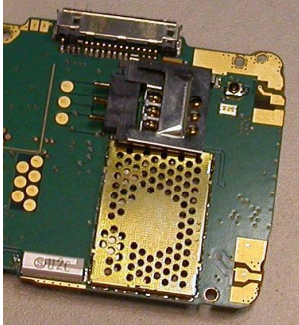
Figure 78 The shield lid in place
