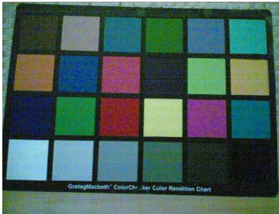
Figure 82 Noisy image taken in +70 degrees Celsius
