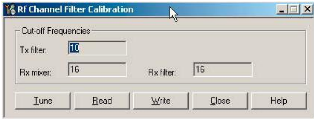
Figure 69 RF channel filter calibration typical values
