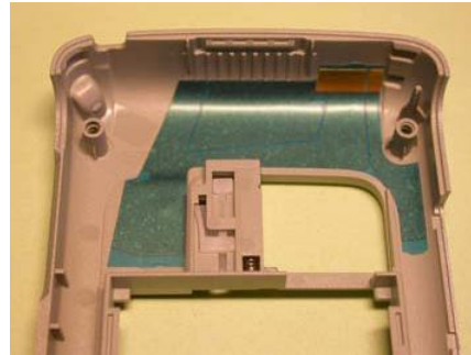
Figure 68 GSM antenna radiator
